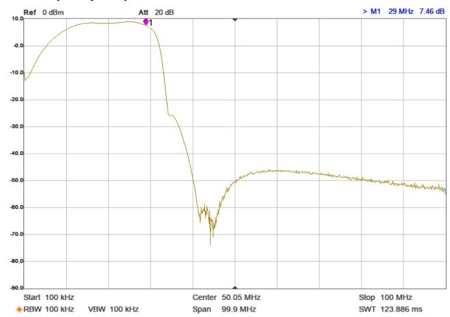
The filter/preamp provides about +9 dB gain between 14 and 28 MHz, with the gain dropping to -10 dB at 1 MHz when both shelf filters are enabled. The attenuation above 40 MHz is around -50 dB or better.
