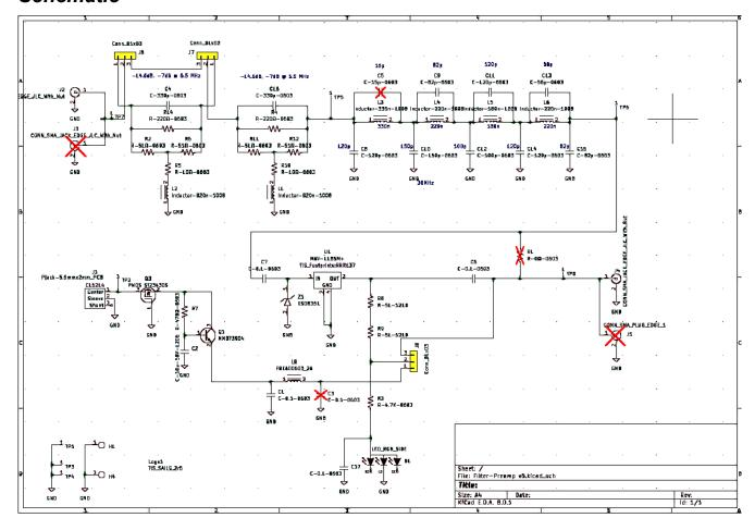
This design has a two-stage high-pass shelf filter (one stage bypassable), followed by a four-section elliptic low-pass filter. The shelf filters provides attenuation at the lower frequencies, reducing the potential overload from AM broadcast-band stations in the USA. This filter will have little effect on European HF broadcast-band signals. The low-pass filter has a sharp cutoff above 30 MHz, greatly reducing SDR sampling aliasing of signals above this frequency.
