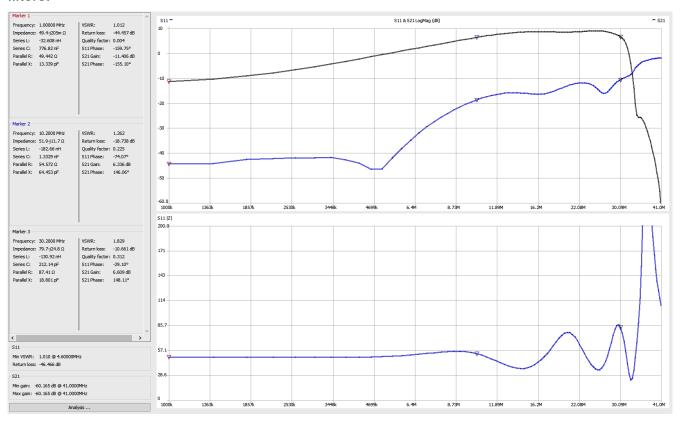
Note that when powering the unit with the remote bias-tee, the amplifier gain will increase about 1dB.
