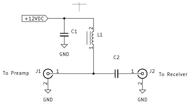
For operation from 1 to 50 MHz, C1 and C2 can be 0.1uF ceramic capacitors, and L1 might be about 22uH.
