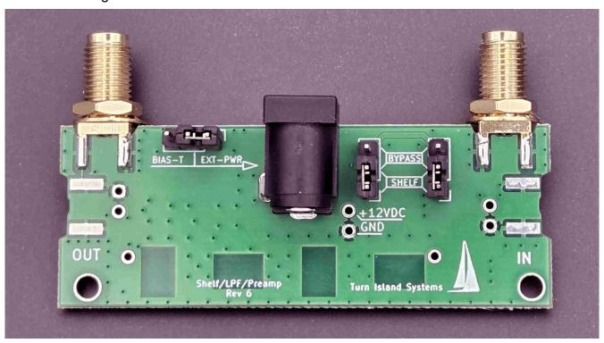
The shelf filter selection jumpers are on the right side of the board. To bypass the shelf filter, move *both* jumpers to the "BYPASS" position.
