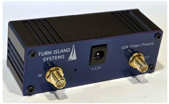
This has the same internal circuit board, but uses an extruded aluminum enclosure that requires much less assembly labor.
