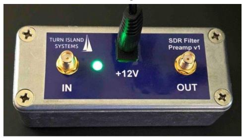
The right-angle-connector filter option fits nicely in a small die-cast enclosure. Here is the filter in a "Hammond 1590A" enclosure, available, custom-milled, as an option from Turn Island Systems. The SMA jacks are on 2-inch centers. While an SMA jack will fit through ¼ inch diameter hole, I suggest making a slightly larger hole to accommodate slight variations in connector alignment.
