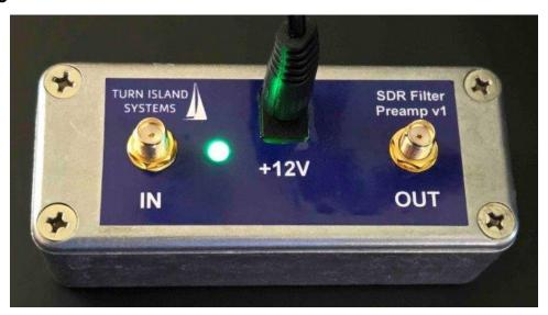
The right-angle-connector filter option fits nicely in a small die-cast enclosure. Here is the filter in a "Hammond 1590A" enclosure, available, custom-milled, as an option from Turn
