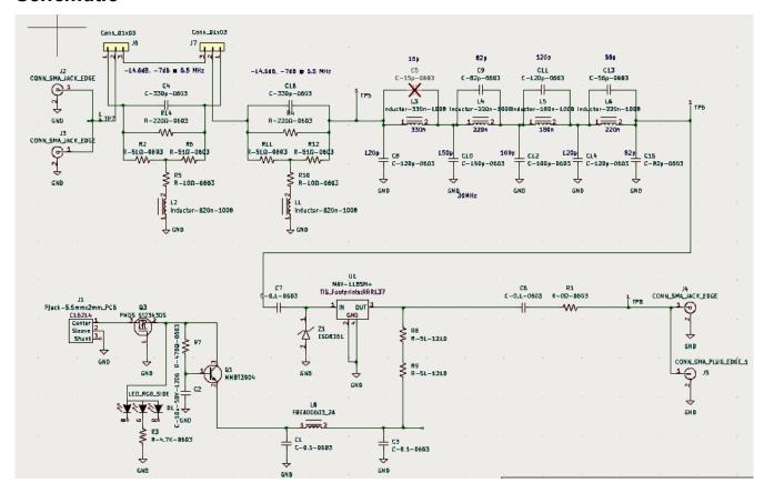
This design has a two-stage high-pass shelf filter (one stage bypassable), followed by a four-section elliptic low-pass filter. The shelf filters provides attenuation at the lower frequencies, reducing the potential overload from AM broadcast-band stations in the USA. This filter will have little effect on European HF broadcast-band signals. The low-pass filter has a sharp cutoff above 30 MHz, greatly reducing SDR sampling aliasing of signals above this frequency.
