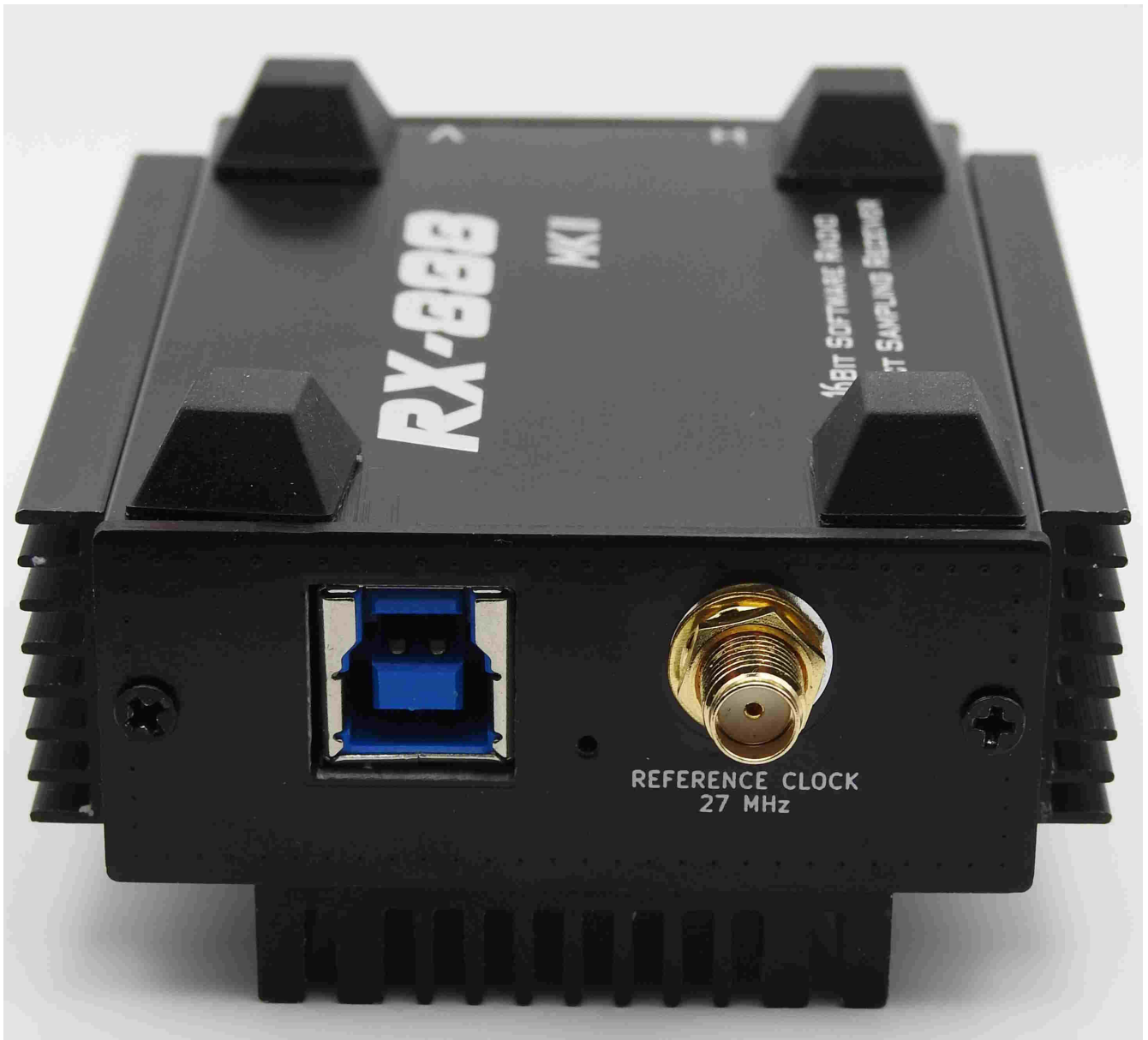
Illustration 4: RX-888 With Replacement Back-Panel
