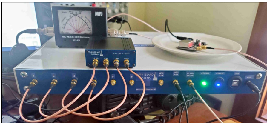
Figure 2. The 'Beacon-Blaster-6' prototype #2 from Turn Island Systems, capable of simultaneous FSK transmissions on six bands from 1.8 MHz to 50 MHz. Image from https://turnislandsystems.com/beaconblaster-progress/
